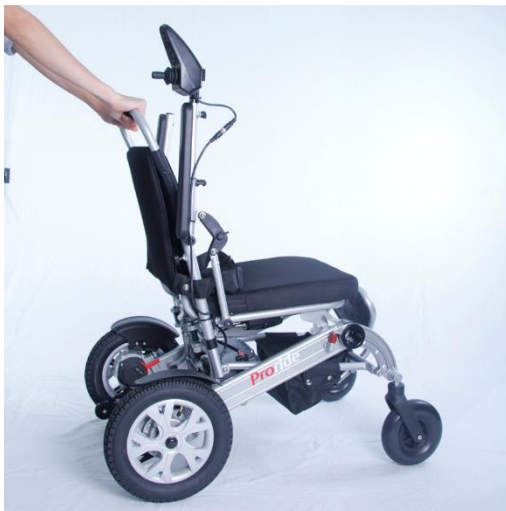
Continue pull the handle until the latch lock itself
